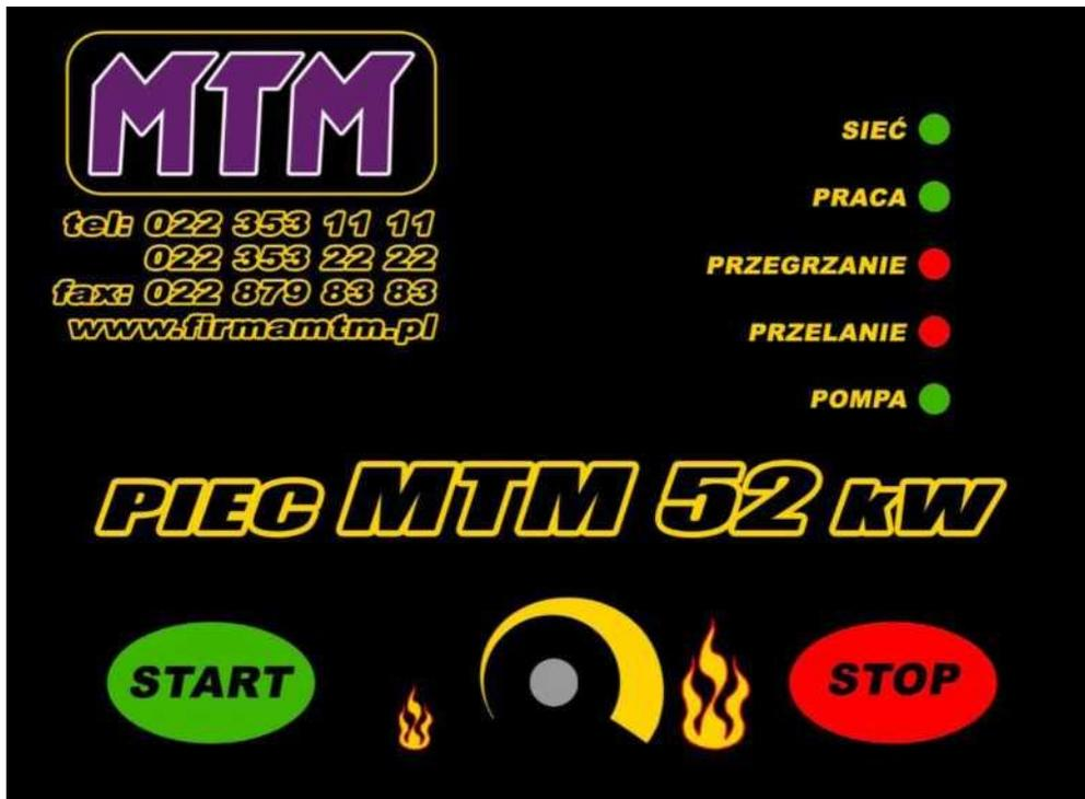
Fig. 4. The front panel of the control module of the universal oil heater.
