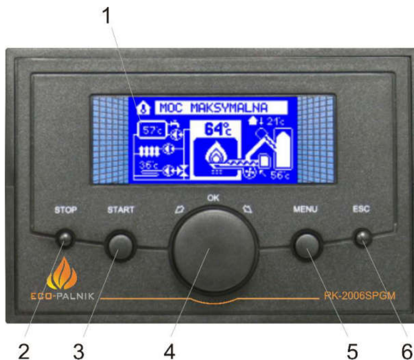
Rysunek 1. Face plate of RK-2006LPG2 controller.
